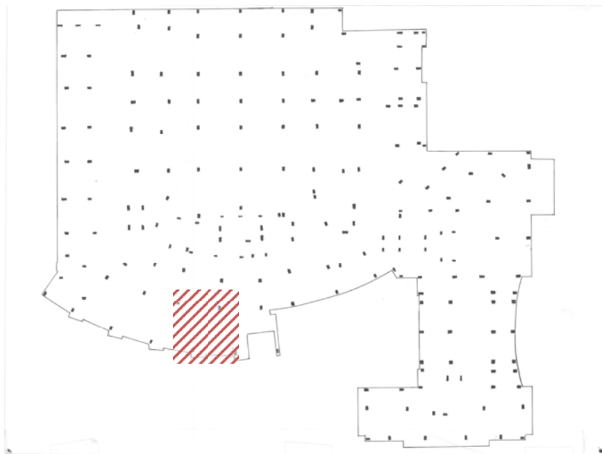
Figure 8: Column layout for the Silver Spring Gateway with the red hatch indicating the area of schematic design.
